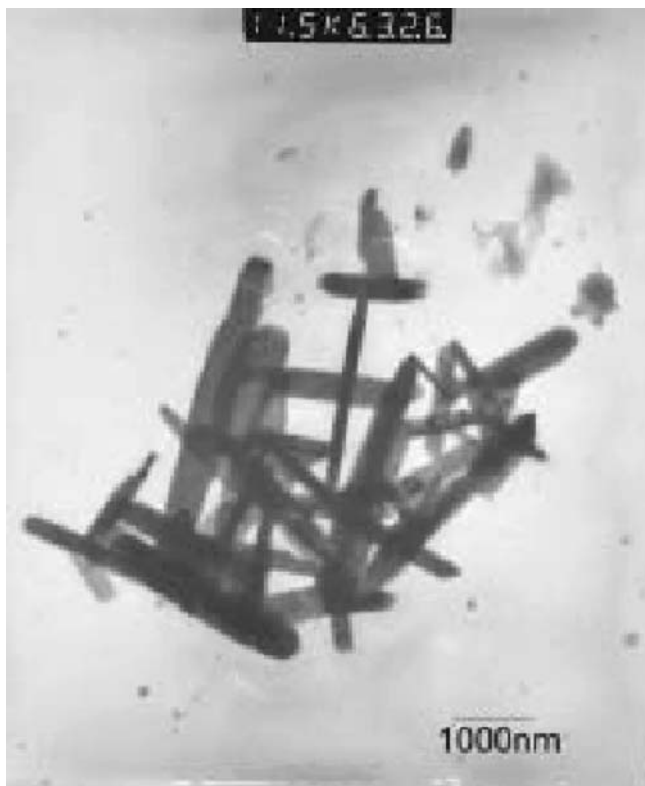
Fig. 7 Transmission electron microscope image of rod-shaped PbS crystals precipitate in the electrolyte solution after the reaction in 0.03 M sodium thiosulfate, 0.1 M sodium sulfate, and 0.01 M TG aqueous solution under stirring for 4 h
